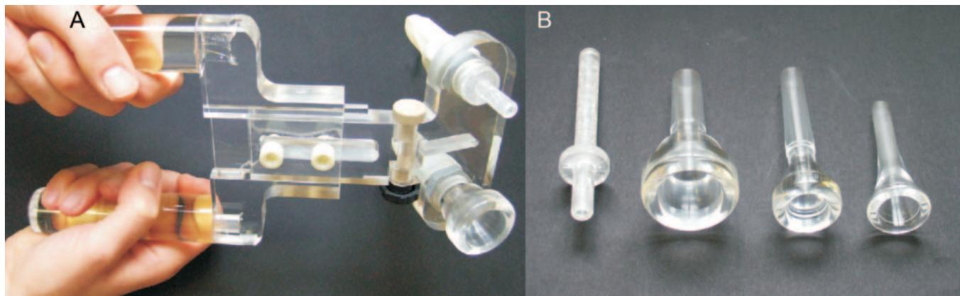
(A) The acrylic glass handhold with mounted mouthpiece and tube and an incised latex finger stall attached to the outlet of each for producing a comparable resistance. (B) From left to right: acrylic glass tube and instrument-specific mouthpieces for trombone, trumpet, and French horn.
